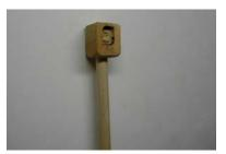
I also decided to make a permanent lightswitcher for the light in their room. I took a different rod and drilled a hole in the end. Then we put grass trimmer line through the hole in the rod. My dad helped me carefully drill a hole in the light switch knob. We put the line through the hole and used a wire end cap to hold the line together to make a loop.
